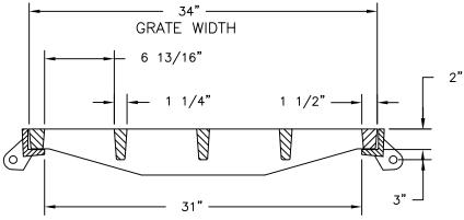
CAUTION: DO NOT DISASSEMBLE BOLTED GRATES AND CHECK <u>FRAME WIDTH INSIDE</u> BEFORE SETTING SECTIONS IN CONCRETE.
